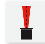
Reflector 0% scat Y10% = 2 x 6,6° Y50% = 2 x 3,6°
