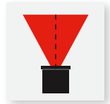
Reflector 20% scat Y10% = 2 x 22,6° Y50% = 2 x 13°
